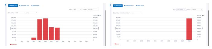
**2.4.2 Multimeter Sum**: This section displays energy consumption data on a daily, weekly, monthly, yearly, and 10-year basis. Users can filter and view the data for specific dates or months as needed, and can also select multiple meters to compare their data side by side.
