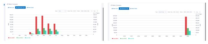
**2.4.3 Meter Detail**: This section displays energy consumption data on a daily, weekly, monthly, yearly, and 10-year basis. Users can filter and view the data for specific dates or months as needed, and can also select multiple meters to compare their data side by side. The results are shown in a stacked chart format, making it easy to clearly see the differences in energy usage.
