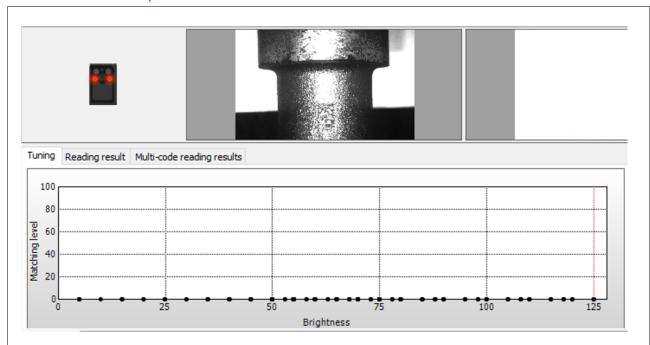
The problem of reading Serial part error is caused by the SR-X300 camera's reading being unable to read. Due to problems with tuning We'll be in touch with Keyence to help with tuning again next week.
