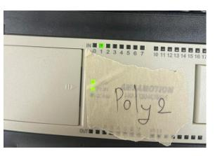
• Example: Connect error signal to plc Mitsubishi in channel IN1. When CVX sends signal to IN1, the light will be on.
